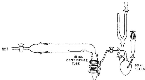
Fig. 1.—Acid generation unit and bromination vessel with condenser separated.
